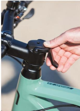
You can prevent any movement by tightening the stem bolts and the handlebar clamp with an Allen key.
